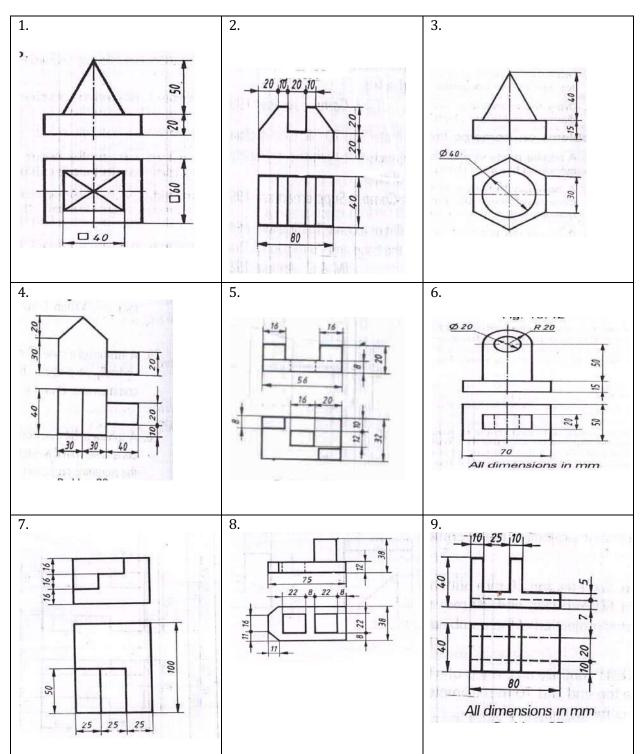
1. .Draw the isometric view of the machine component whose orthographic views are given below:
